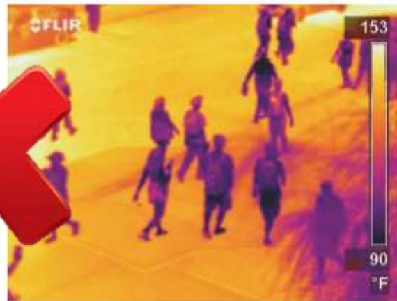
This picture of Phoenix, Arizona, in the summer shows a variety of conventional pavements that reached temperatures up to 150°F (67°C).
